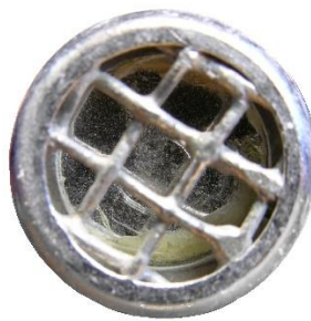
2. Good condition. Glue is visible on the foil edge, and there are some foil scratches from when the foil was manufactured
