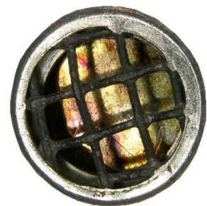
3. Poor condition. The foil is discoloured. The source passed its leak test, but it should be disposed of
